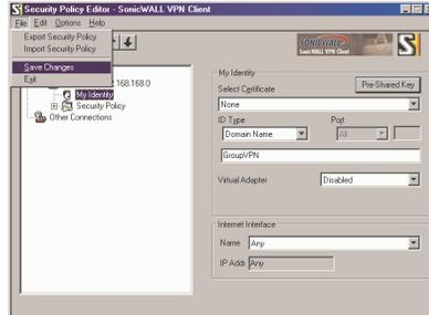
It is not necessary to configure the **Security Policy** as it is imported directly into the **Client** application. Exporting the security association to a file facilitates configuration of a large number of VPN clients and you do not have to configure each client individually. You can distribute multiple copies of the configuration file via floppy disk or other distribution means.
